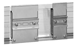
SLZ11-14 adapters allow mounting PULS switched mode power supplies or other DIN rail units on the S7-300 rail, which differs from other rails. Thus, a separate DIN rail is not necessary anymore. The adapter consists of a mounting bracket which is put onto the S7-300 rail and fixed at the lower edge with two
